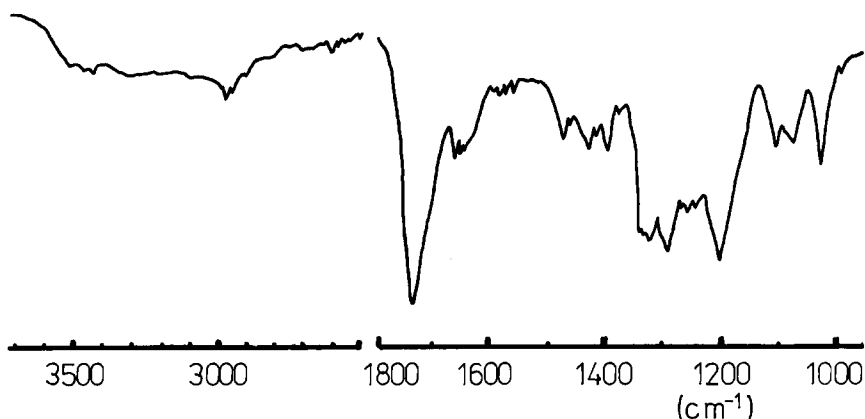
Figure 4. Infrared spectrum of gelled polyester
